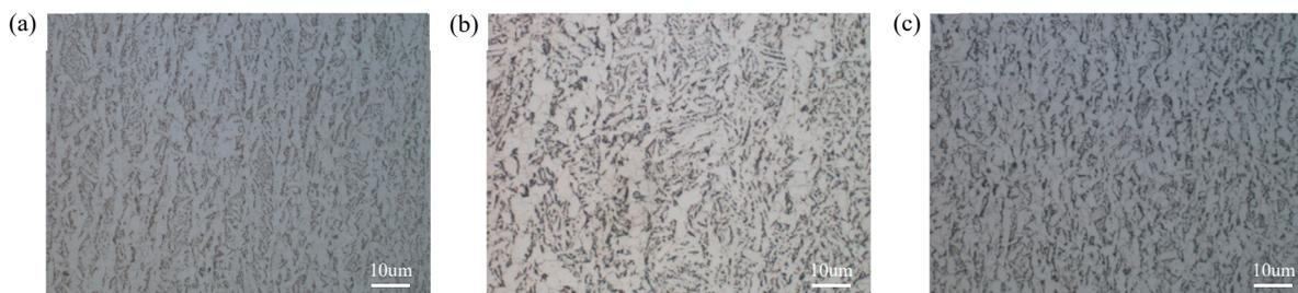
Figure 4. OM images on 1/4 length sections of E36 (a), EH36 (b) and FH36 (c) steel plates.
