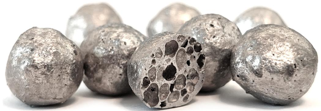
**Figure 1.** Advanced pore morphology foam elements.
