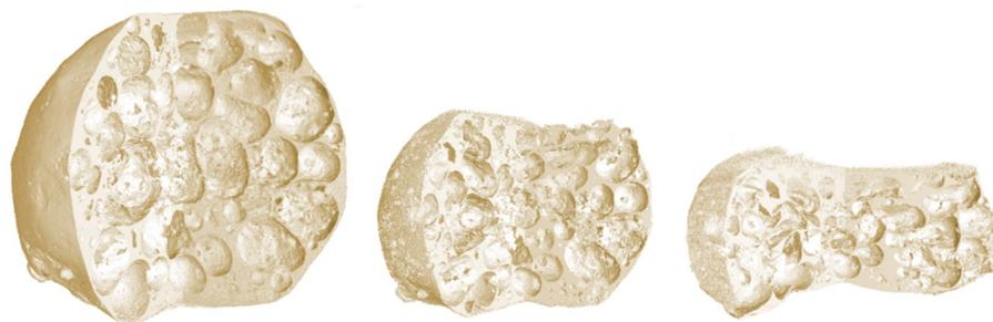
**Figure 3.** Visualisation of a deformed APM sphere—reconstructed 3D image captured after loading steps 1, 13 and 25.
