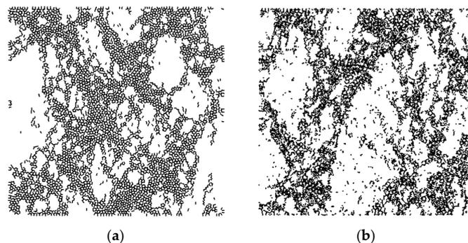
**Figure 9.** Simulation compression failure diagram of concrete. (a) Ordinary concrete. (b) Nano-TiO<sub>2</sub> modified concrete.
