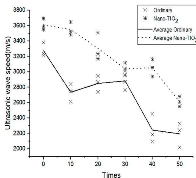
**Figure 3.** The influence of dry–wet cycles on the concrete ultrasonic wave velocity.
