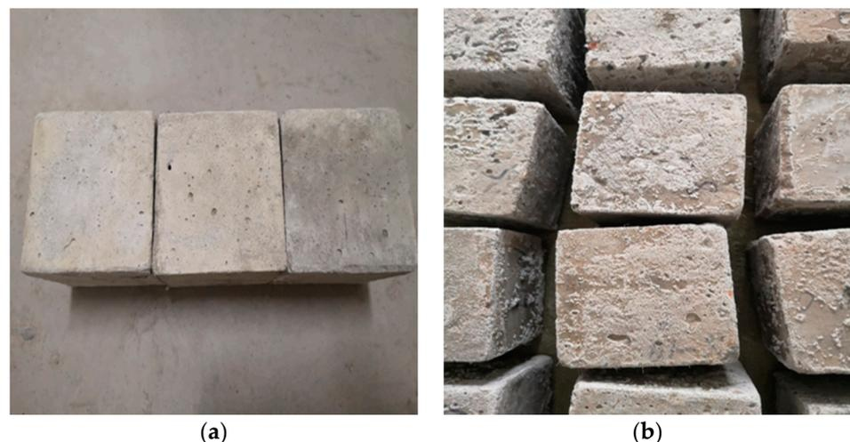
**Figure 1.** Nano-TiO<sub>2</sub> modified concrete specimen. (a) Specimen at room temperature. (b) Specimen after dry–wet cycle.
