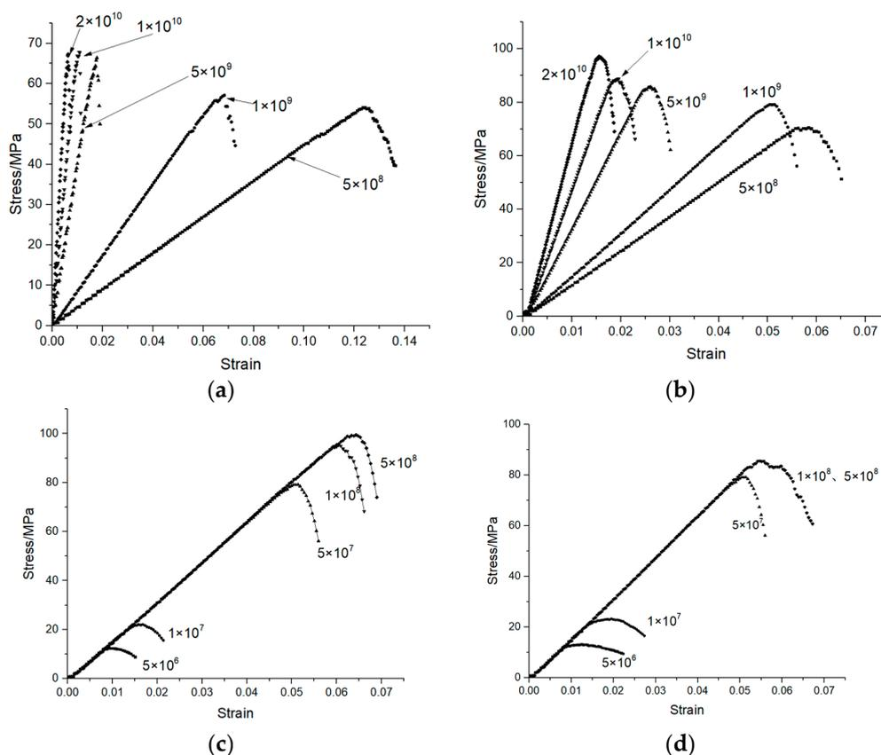
**Figure 7.** The influence of four main parameters on compressive stress–strain. (a) Pb\_omod. (b) Cb\_omod. (c) Ten. (d) Coh.
