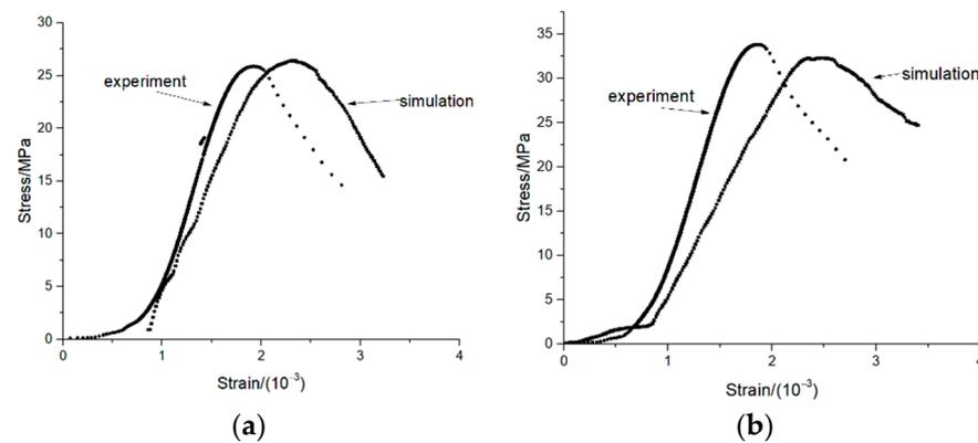
**Figure 10.** Test and simulated stress–strain diagram of specimens. (a) Ordinary concrete. (b) Nano-TiO<sub>2</sub> modified concrete.
