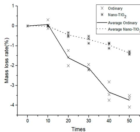
**Figure 2.** The influence of dry–wet cycles on the concrete mass-loss rate.
