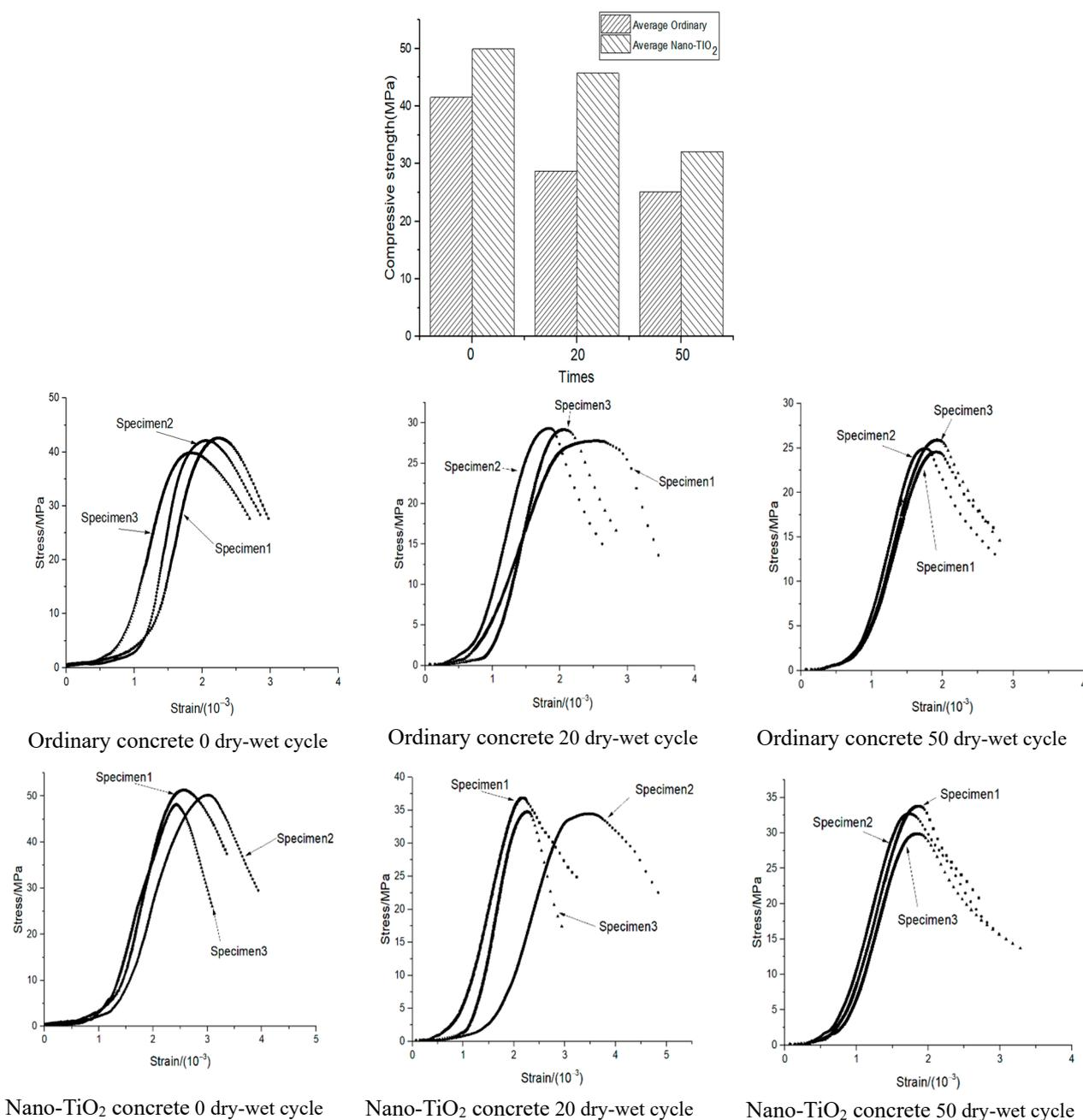
Figure 4. The influence of dry–wet cycles on the concrete compressive strength.
