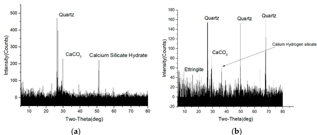
**Figure 5.** Powder diffraction patterns from concrete. (a) Nano-TiO<sub>2</sub> modified concrete at room temperature. (b) Nano-TiO<sub>2</sub> modified concrete after dry-wet cycle.
