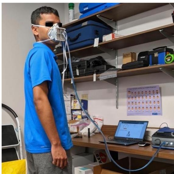
Figure 7. Subject wearing the Moldable Mask during fit testing.
