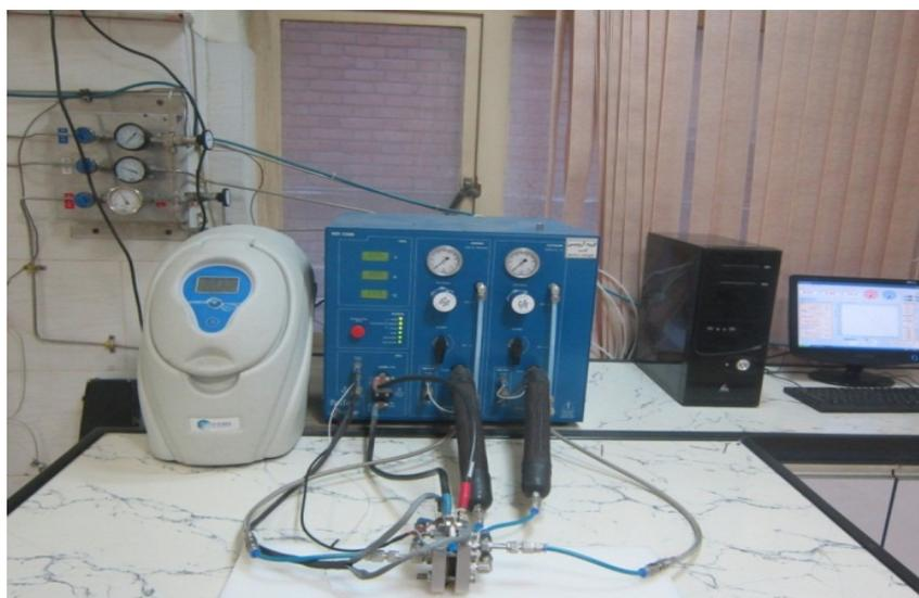
Figure 5. FCT-150s Fuel Cell Station.
