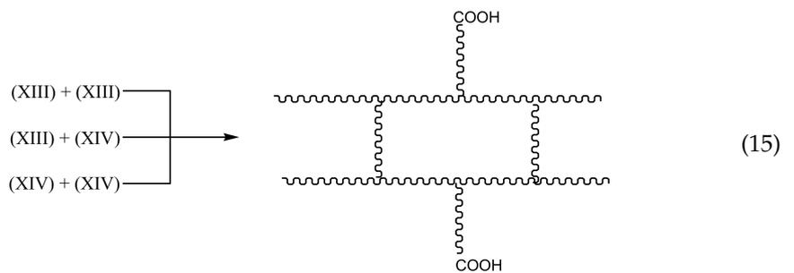
Crosslinking of XNBR using PO:
