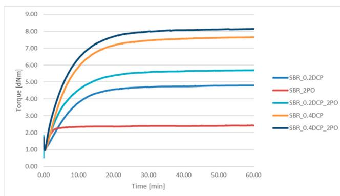
**Figure 2.** Crosslinking kinetics of the compounds based on styrene-butadiene rubber (SBR).
