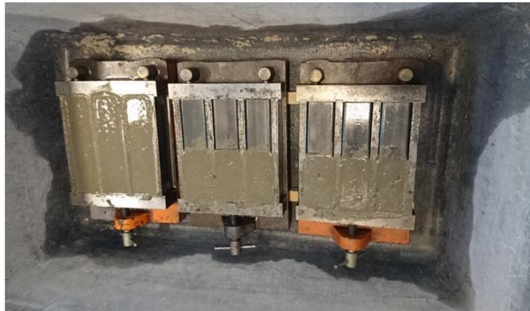
**Figure 2.** An example of a set of moulds filled with cement paste (MCP) mixture for testing at a single age.
