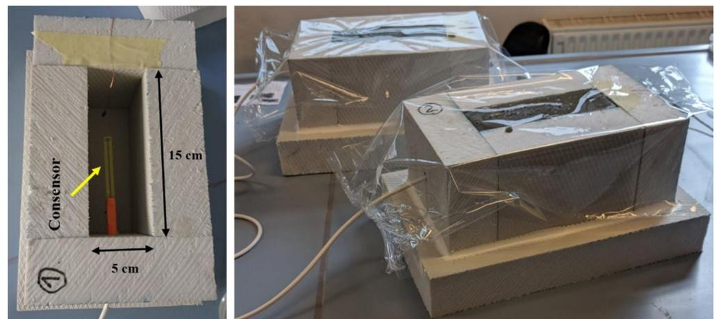
**Figure 3.** Custom-made container (left) and moulded specimens prepared for temperature and conductivity measurements (right).
