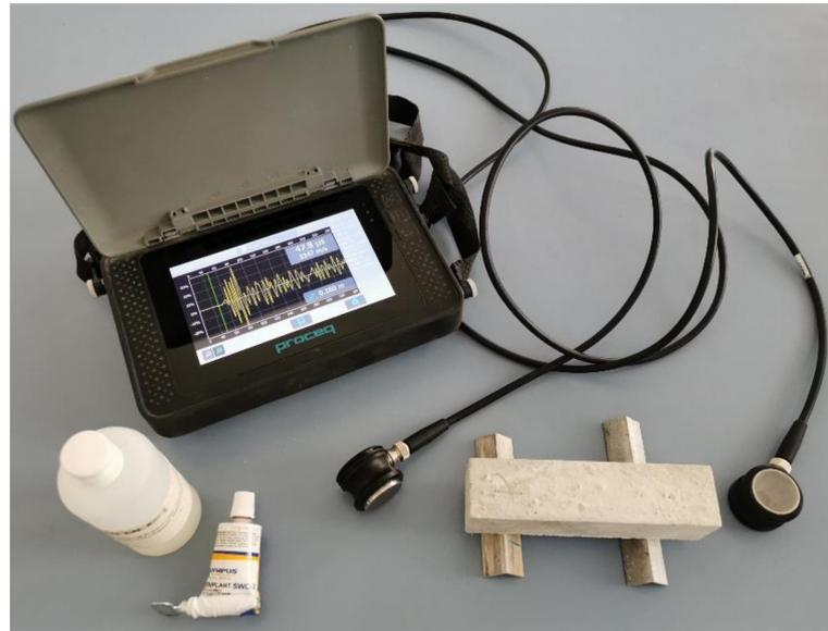
Figure 4. Ultrasonic device Proceq Pundit PL-200.
