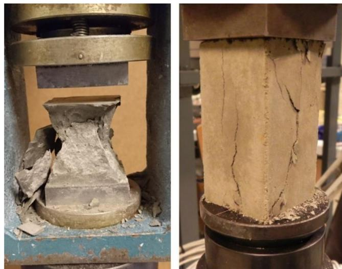
**Figure 6.** An example of MCP cube compression test (left) and MCP prism compression test (right).
