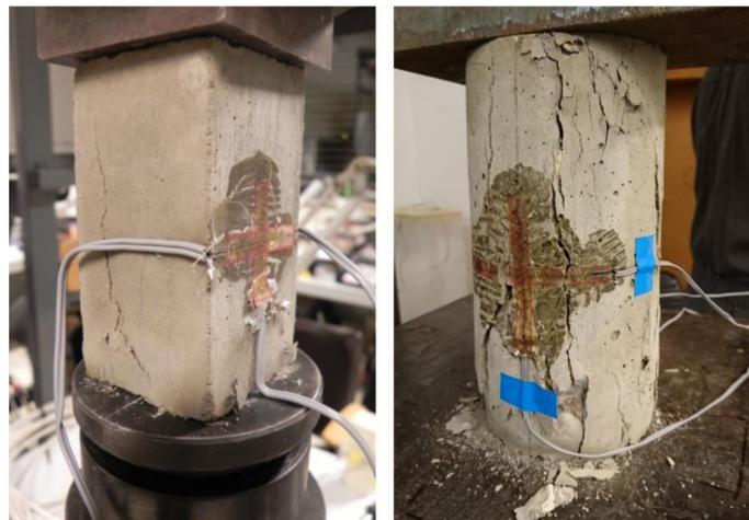
**Figure 7.** An example of a prism specimen of MCP/ mortar (MOM) (left) and cylinder specimen of concrete (MOC) (right) after the modulus of elasticity, Poisson's ratio and  $\sigma$ - $\varepsilon$  test.
