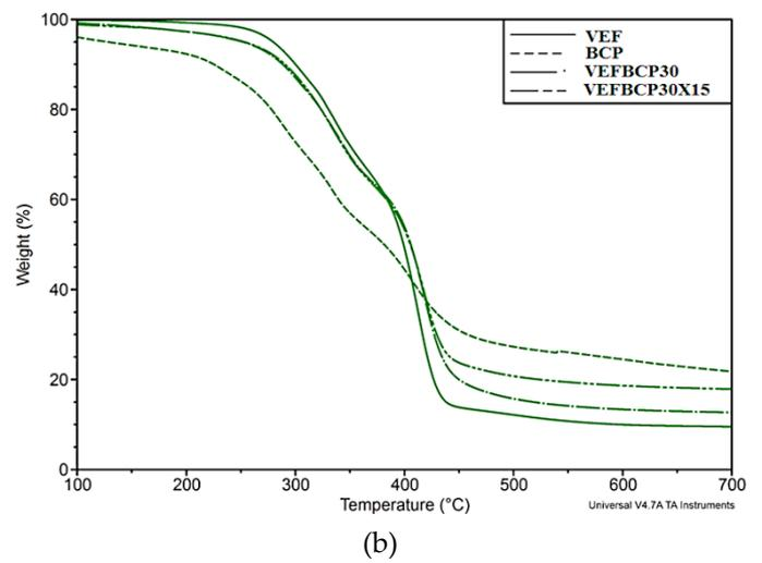
**Figure S1.** TG curves for VEF foams and their composites containing: **(a)** different amounts of EG L, **(b)** BCP and a mixture of BCP and EG X.
