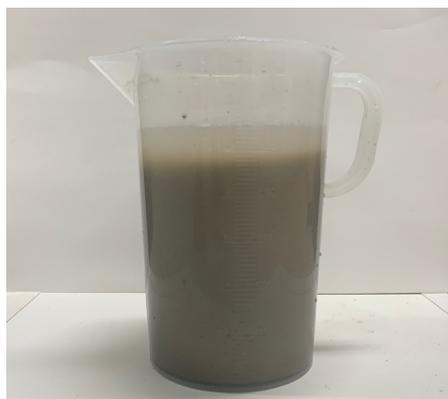
**Figure 4.** Concrete slurry water.
