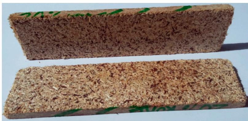
**Figure 10.** Particleboard specimens before bending test.
