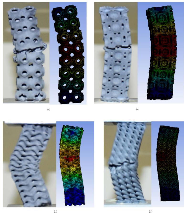
**Figure 13.** Numerical and experimental patterns of buckling behavior for uniaxial compressive samples of various morphologies. The figures reveal that the experimental and FEA results show good agreement. Samples with  $2 \times 2 \times 8$  configuration: (a) Schwarz-P, (b) Neovius, (c) Gyroid and (d) Diamond.
