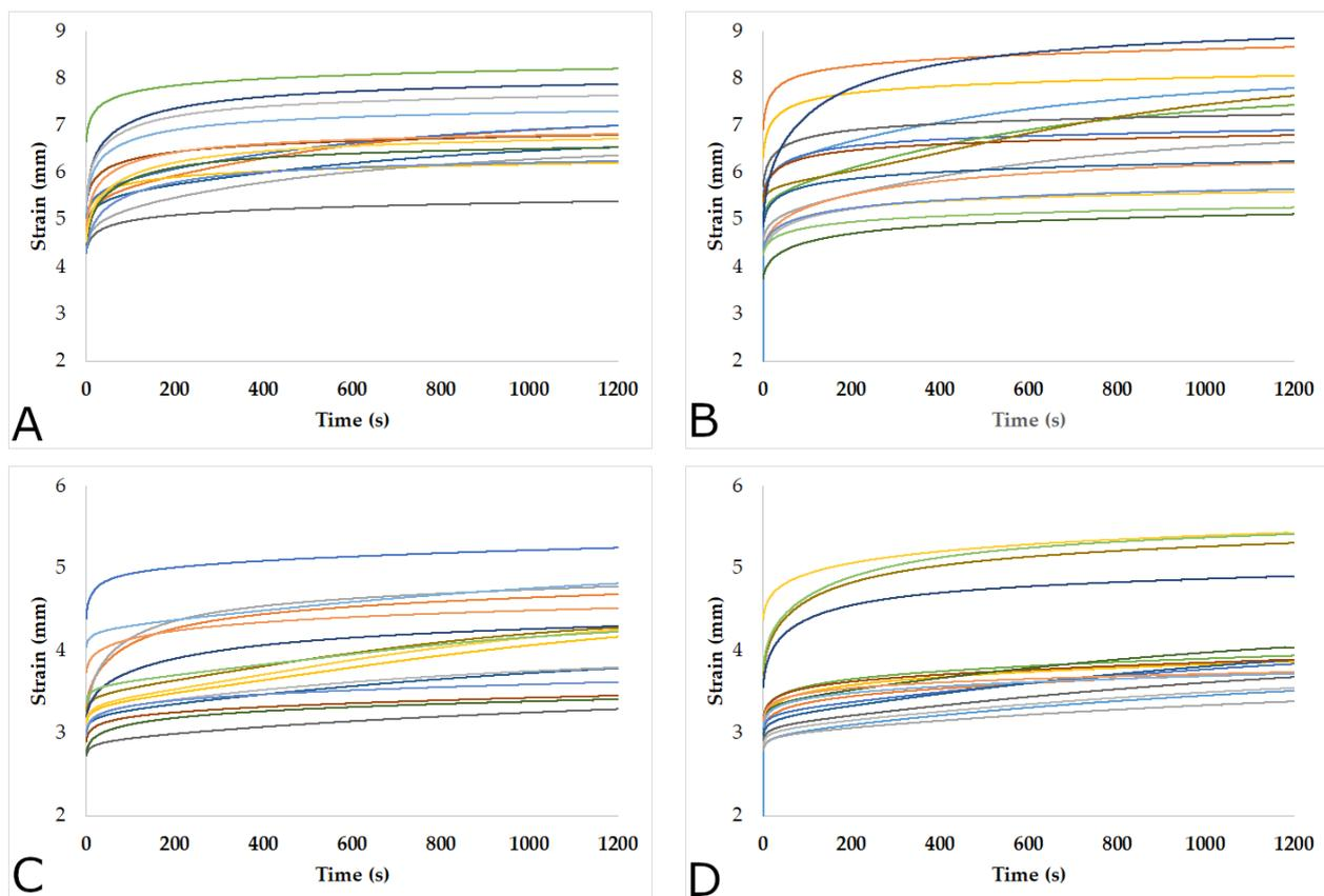
**Figure 4.** Evolution of the pieces with a density of  $0.39 \text{ g cm}^{-3}$  subjected to tensile creep: Load 1530 N: (A) tangential; (B) radial. Load 1170 N: (C) tangential; (D) radial.
