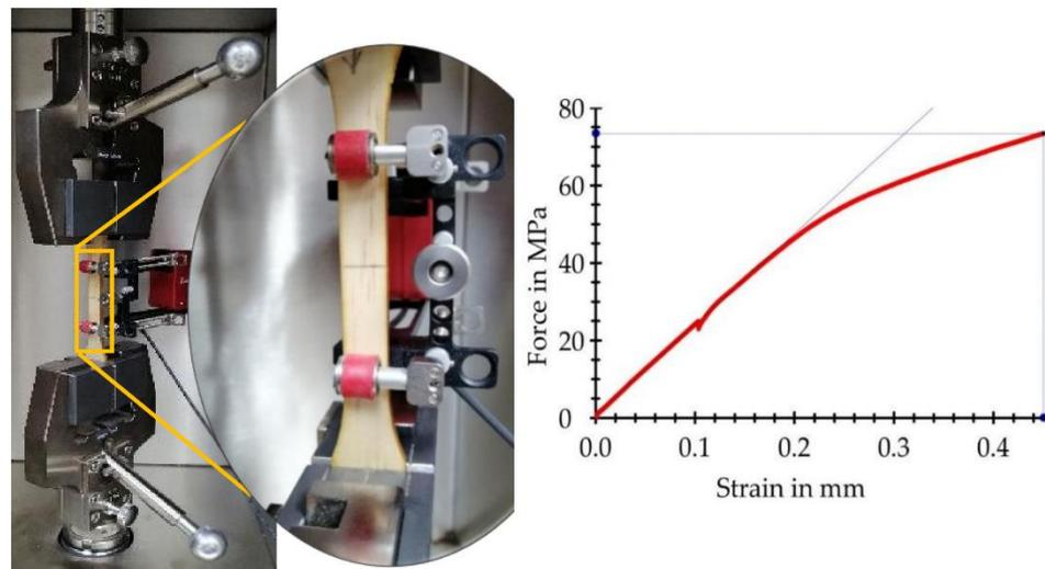
**Figure 2.** Clip-on extensometer. Determination of the force at the proportional limit.
