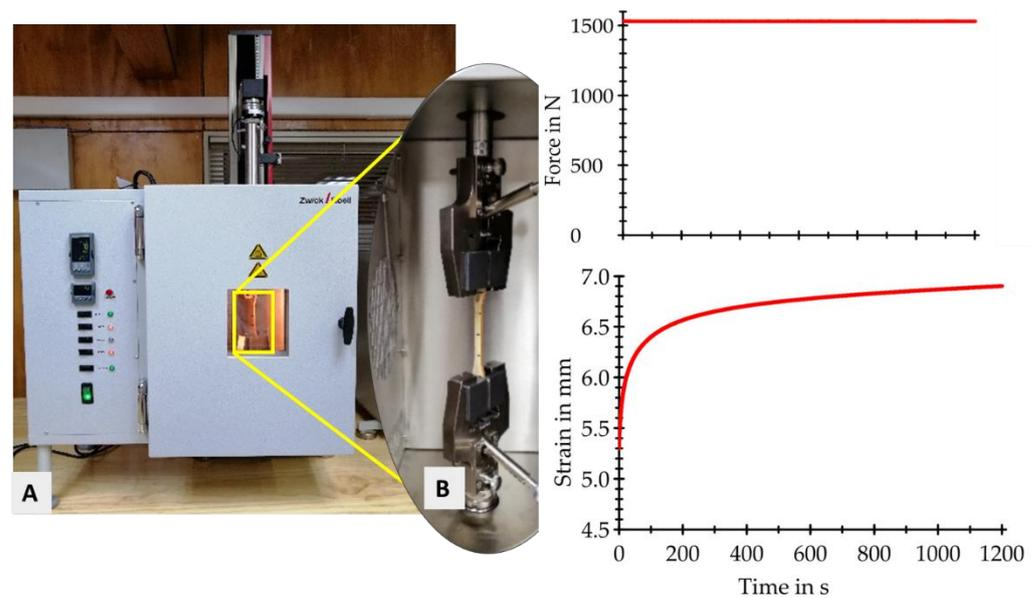
**Figure 3.** Tensile creep test: (A) testing machine equipped with temperature chamber; (B) specimen during tensile creep test.
