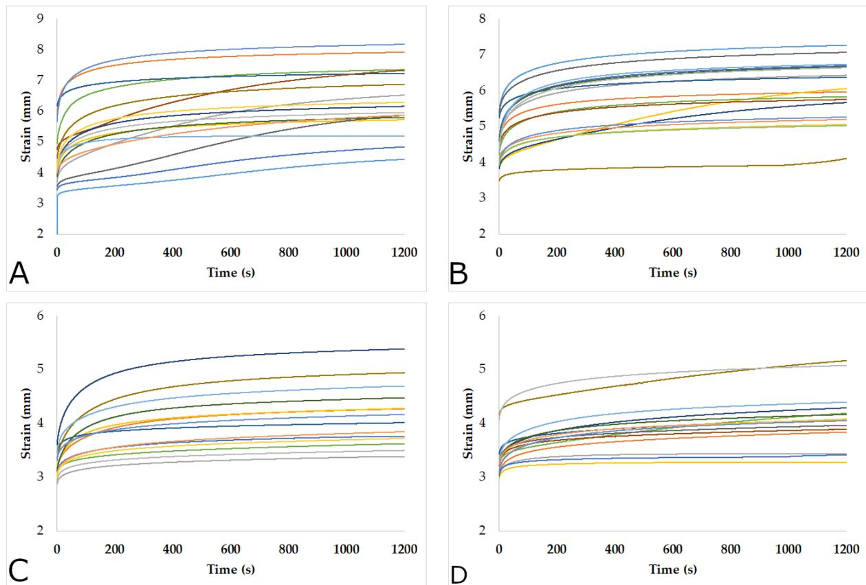
**Figure 5.** Evolution of the pieces with a density of  $0.43 \text{ g cm}^{-3}$  subjected to tensile creep: Load 1530 N: (A) tangential; (B) radial. Load 1170 N: (C) tangential; (D) radial.
