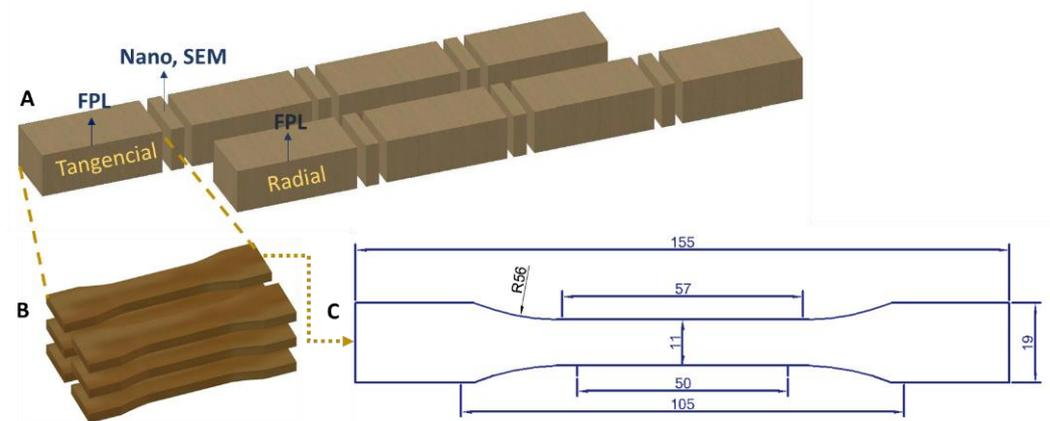
**Figure 1.** Diagram for obtaining the specimens in a strip: (A) sections in a wooden strip: tangential and radial; (B) dog bone specimens per section; (C) dimensions in millimeters (mm) of the dog bone specimen.
