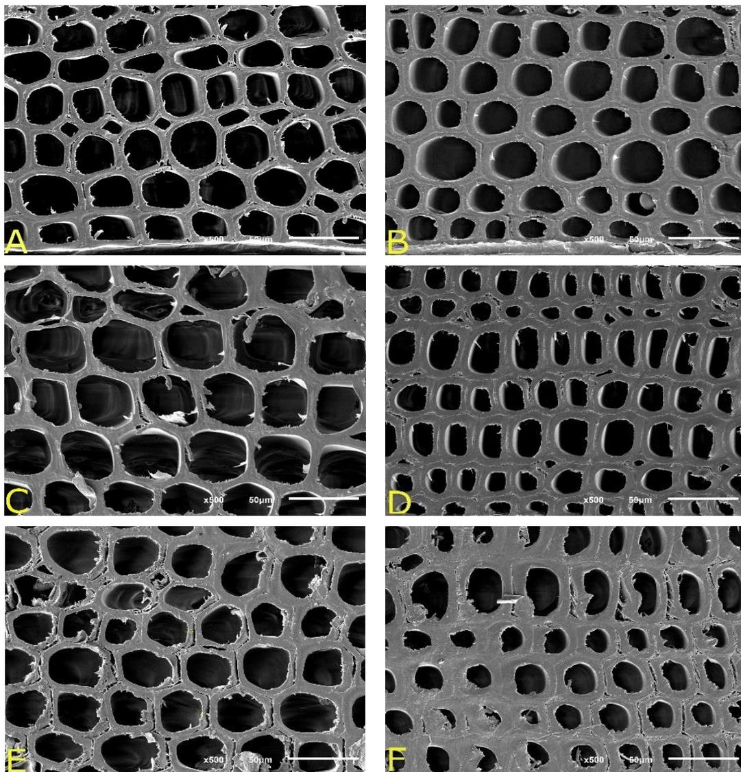
**Figure 6.** SEM images of radiata pine wood samples: untreated (A) earlywood (EW); (B) latewood (LW). Samples subjected to tensile creep: (C) EW section of a piece loaded 1170 N; (D) LW section of a piece loaded 1170 N; (E) EW section of a piece loaded 1530 N; (F) LW section of a piece loaded 1530 N.
