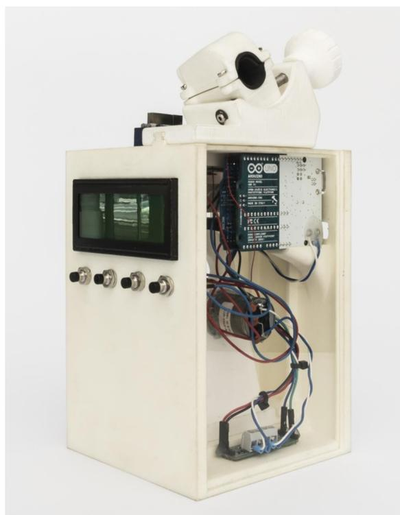
**Figure 1.** Design of prototype based on 2D/3D CAE (computer-aided engineering) (Midas FX, Brunleys, Milton Keynes, UK) software and parts of the hardware of the cyclic fatigue test device.
