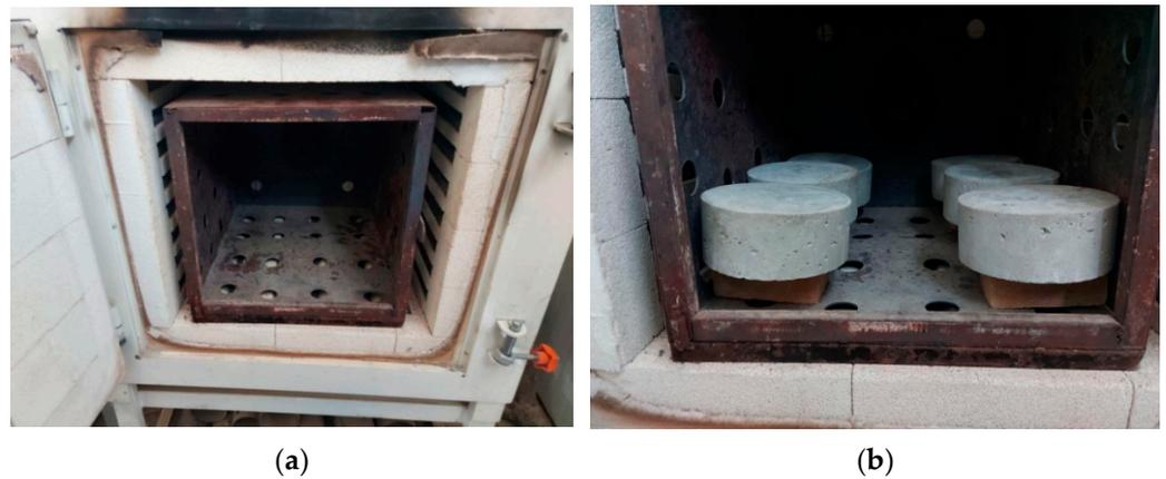
**Figure 2.** Heating of test specimens: (a) the used electrical furnace; (b) specimen heating.
