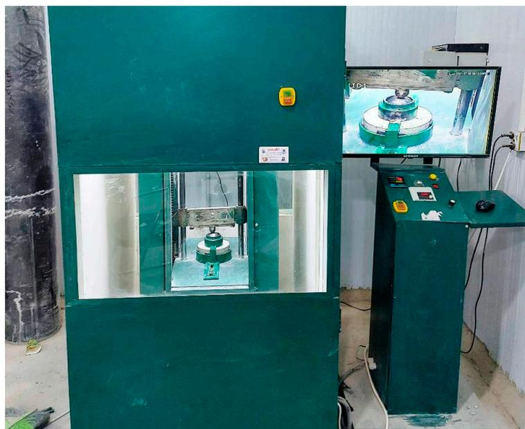
**Figure 5.** The repeated impact automatic testing machine.
