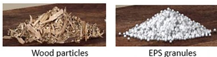
Figure 1. Wood particles and EPS granules used for manufacture of lightweight particleboards.
