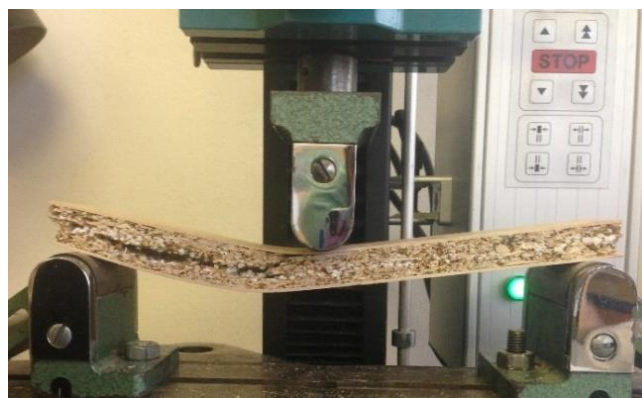
Figure 5. Delamination of the samples under bending strength test.
