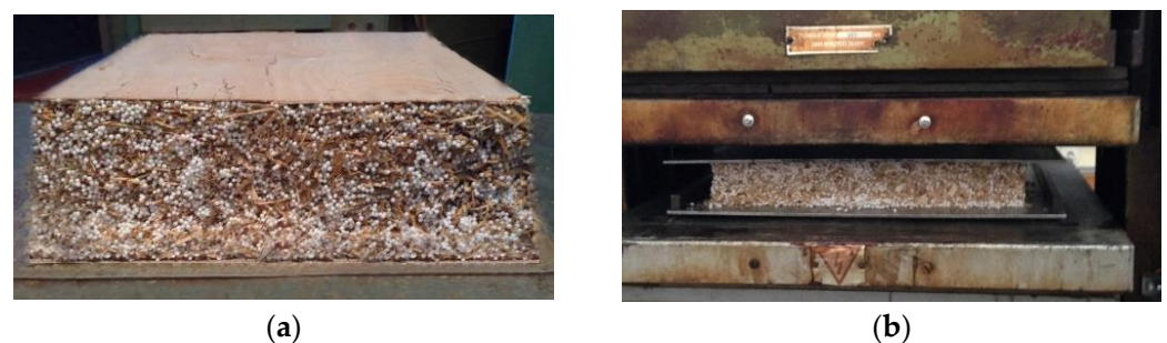
Figure 3. Pre-pressed mat (a) and the board pressing in the hot press (b).
