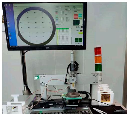
**Figure 2.** MT200 frequency tester.
