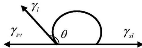
Figure 6. Schematic diagram of interface between the reagent and limestone.
