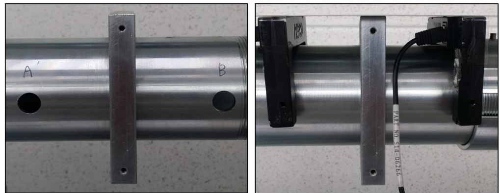
Figure 22. Photogate installed on the SHPB apparatus.
