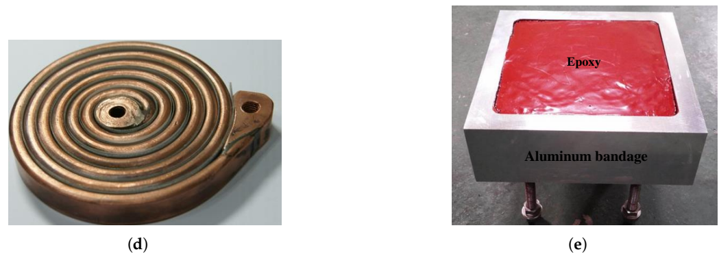
Figure 5. Experimental set up for EMF free bulge test. (a) Forming coil with a test bed. (b) Forming die. (c) Cross-section of a forming die. (d) Forming coil. (e) Insulation block.
