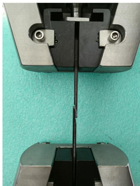
**Figure 4.** Tensile shear test of single-lap specimen.
