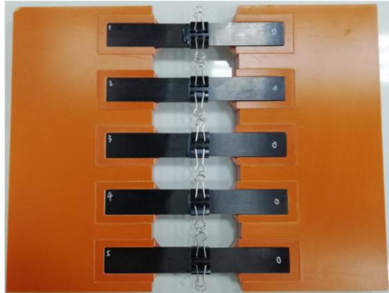
**Figure 3.** The fabricated single-lap specimen.
