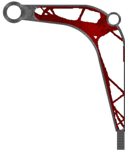
**Figure 23.** The final topology found for the control arm.
