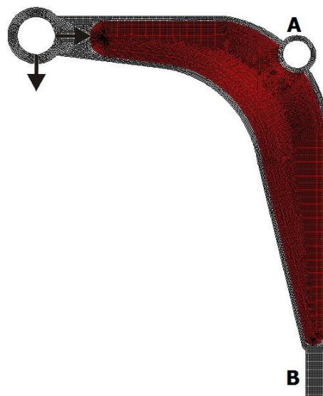
**Figure 22.** The design domain, loads, and supports of the control arm.
