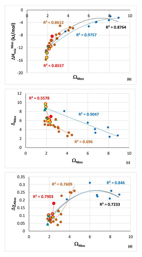
**Figure 2.** (a) Alloy entropy of mixing versus solid solution entropy of mixing, and (b-d) relationships of the solid solution parameter  $\Omega$  with the solid solution (b) enthalpy of mixing, (c) parameter  $\delta$
