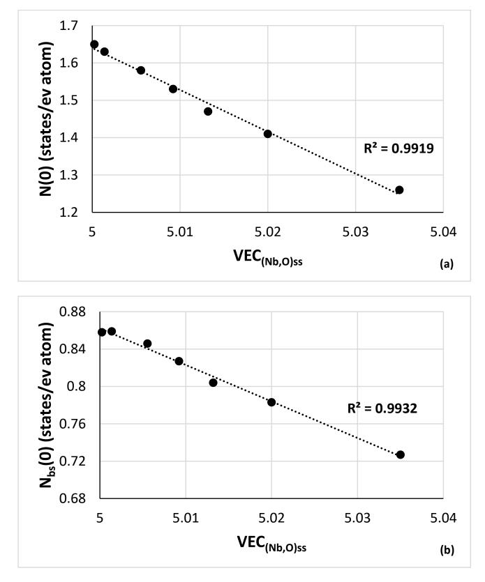
**Figure 13.** Data for Nb contaminated with oxygen. (**a**) density of electronic states at the Fermi level N(0) and (**b**) "band structure" density of states  $N_{bs}(0)$  versus the parameter VEC of the (Nb,O)<sub>ss</sub>.
