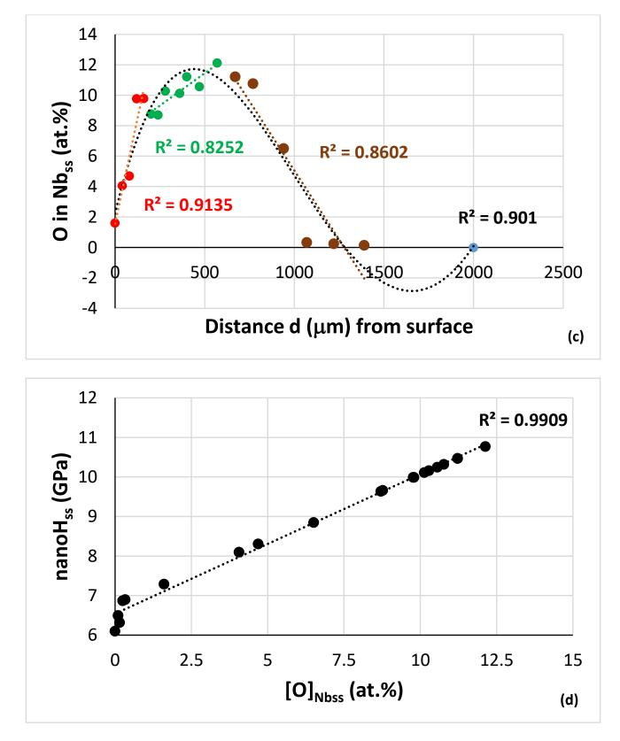
**Figure 12.** (a) Average nanohardness, (b) average Young's modulus and (c) average oxygen concentration of the Nb<sub>ss</sub> in NV1-HT (1500 °C/100 h) as a function of distance from the surface of heat treated specimen. In each part, all the data fit to a 4th order polynomial (see text) with R<sup>2</sup> values 0.921, 0.8968 and 0.9016, respectively, for (**a**–**c**). (**d**) Nanohardness of Nb<sub>ss</sub> versus oxygen content.
