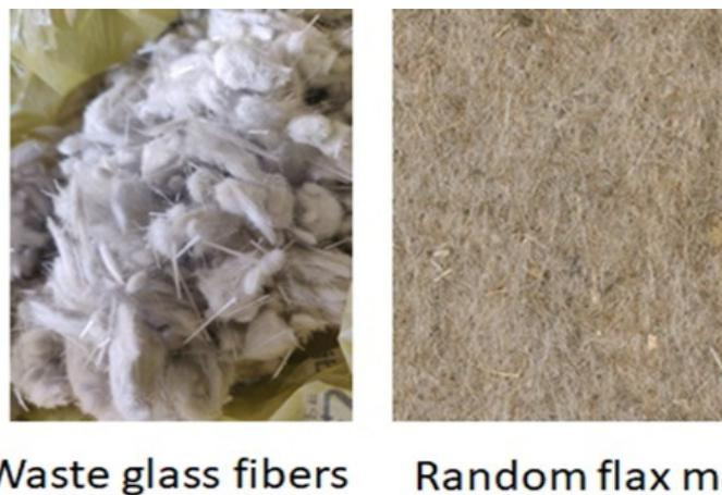
Figure 2. Reinforcements used in this study (left) waste glass fibers and random flax mat (right).
