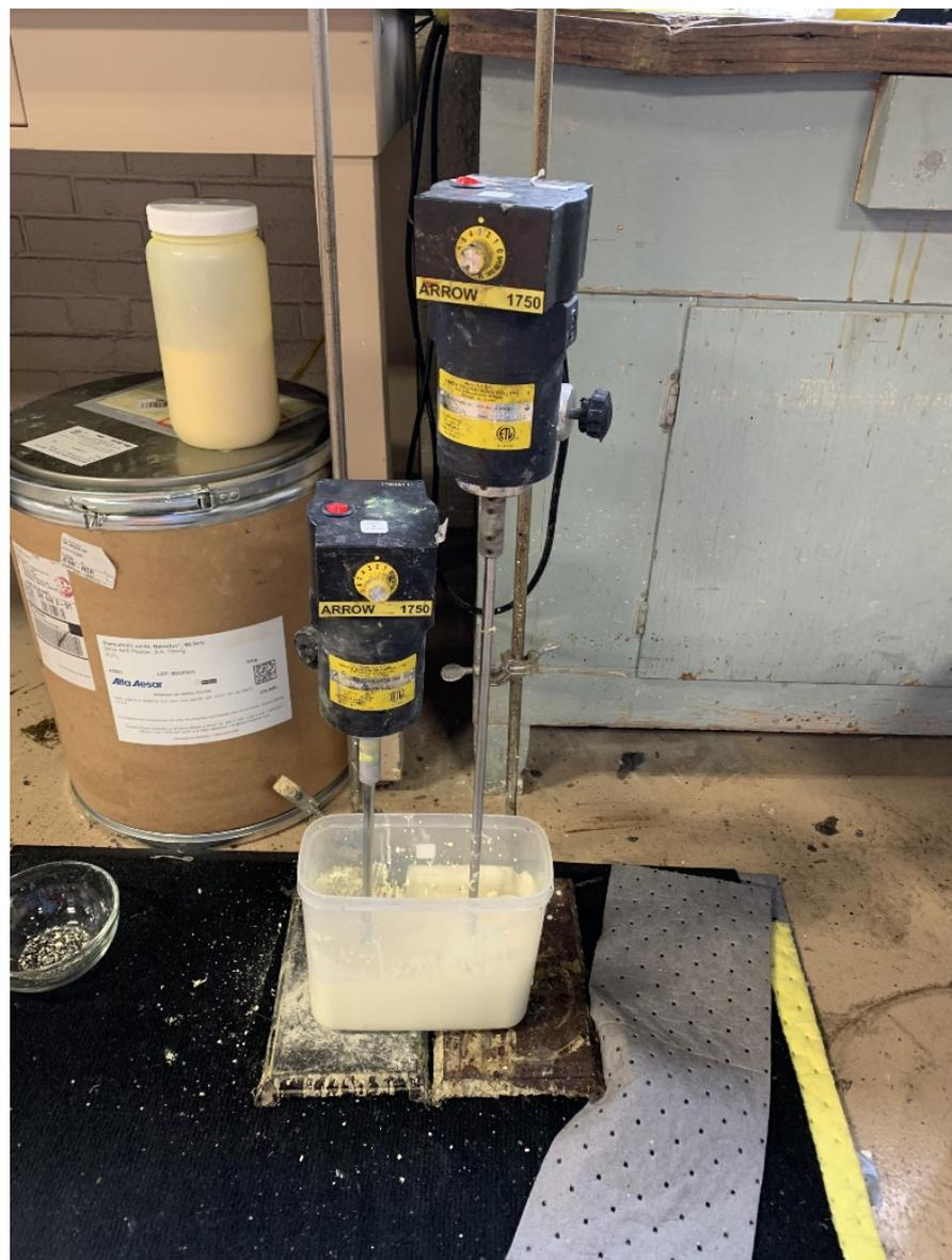
**Figure 1.** Compounding of micro-Bi<sub>2</sub>O<sub>3</sub> in the GNRL.
