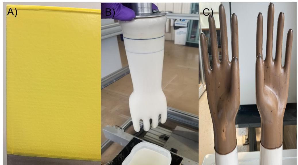
**Figure 2.** Films and RA gloves preparation. (A) Pre-curing of GNRL/micro-Bi<sub>2</sub>O<sub>3</sub> film prepared by dipping; (B) Preparation of glove former before dipping into GNRL/micro-Bi<sub>2</sub>O<sub>3</sub>; (C) Post-curing RA gloves.
