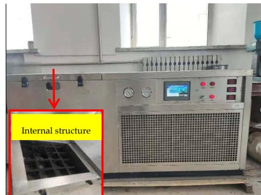
**Figure 2.** Freeze-thaw cycle machine.
