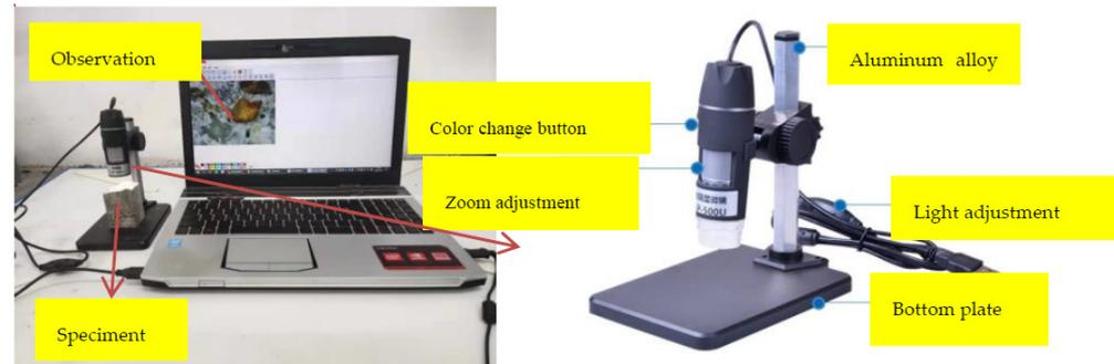
**Figure 4.** Schematic diagram of microscope observation.
