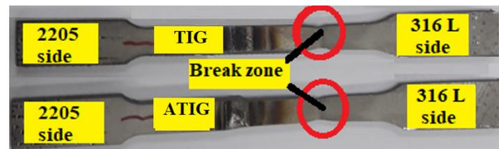
Figure 16. Specimens of the tensile testing after the test.
