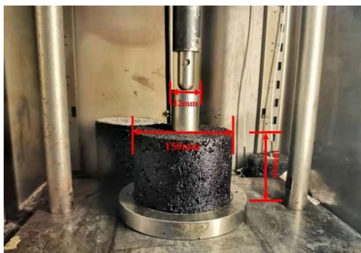
**Figure 5.** Loading device for uniaxial penetration creep test.
