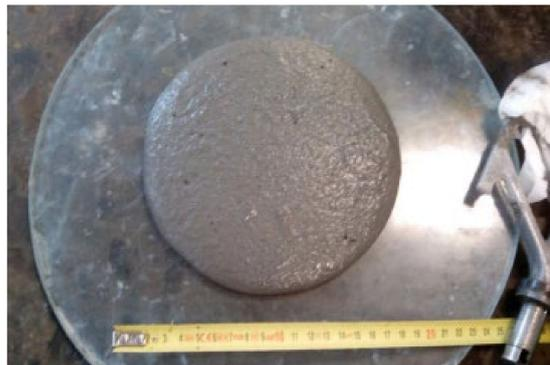
**Figure 4.** Measurement of the stabilized biscuit.
