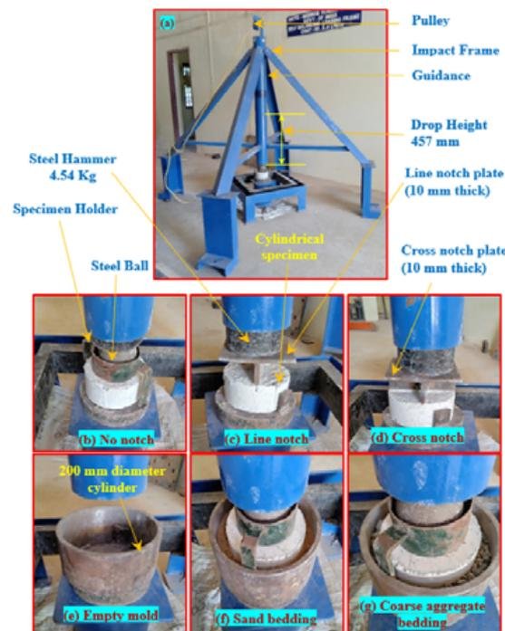
**Figure 7.** Drop weight test setup and arrangements.
