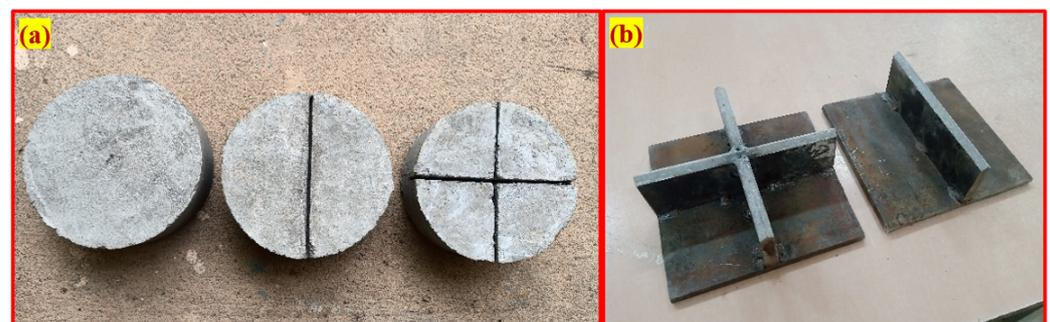
**Figure 2.** Modification details (a) specimens with and without notch (b) load transfer plates.
