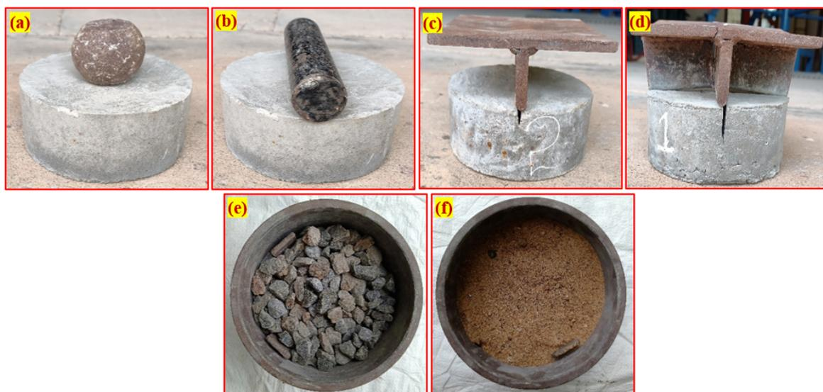
**Figure 3.** Modifications to the ACI test method: (a) ACI method. (b) Line impact load transfer by steel bar. (c) Line notch specimen with load transfer plate. (d) Cross-notch specimen with load transfer plate. (e) Coarse aggregate bedding. (f) Sand bedding.
