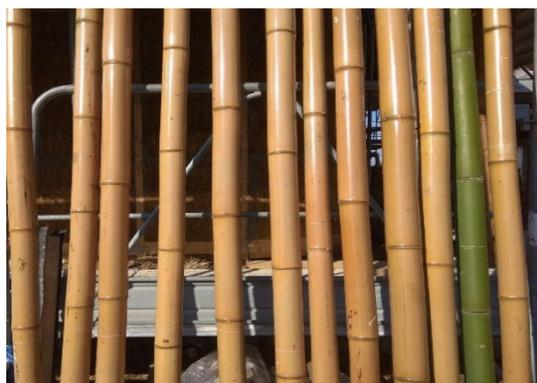
**Figure 2.** Drying of an untreated green culm and several treated ones.
