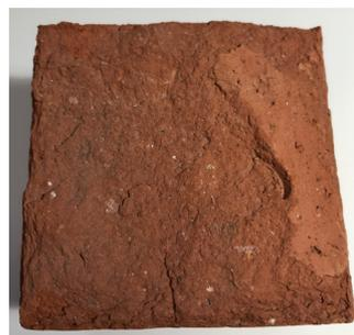
**Figure 13.** Visual inspection of the  $C_W$  samples after 300 freeze–thaw cycles.
