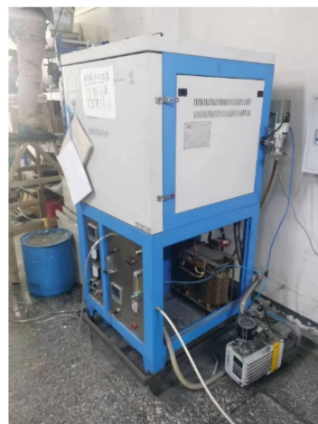
Figure 3. Picture of a self-made nitriding furnace. On the basis of the vacuum sealing furnace, the vacuum pump and nitrogen gas cylinder device are connected.
