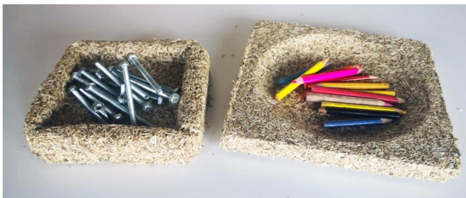
**Figure 13.** Hemp shive material dishes produced in specially created plywood moulds.
