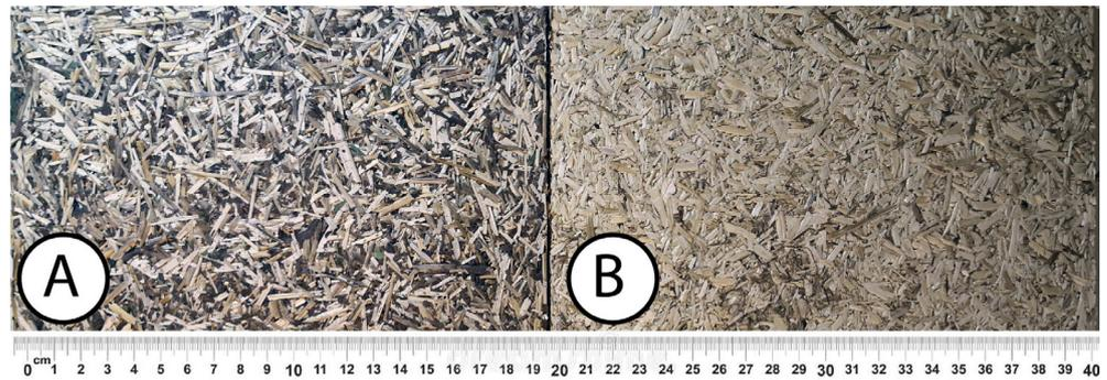
**Figure 7.** (A) Whole hemp stem particle board sample, (B) hemp shive board sample.
