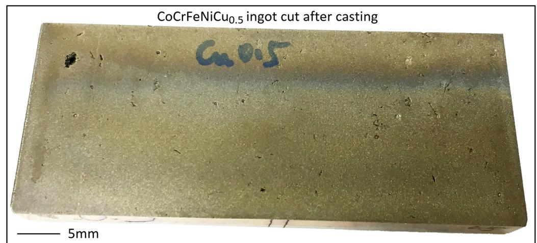
**Figure 2.** CoCrFeNiCu<sub>0.5</sub> ingot showing internal porosity exposed after cutting.
