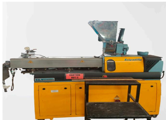
**Figure 6.** Lab Tech Twin Screw Extruder.
