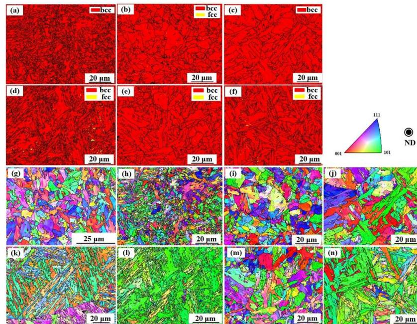
**Figure 5.** Lattice structure in the LCS layer annealed at: (a) 700 °C; (b) 800 °C; (c) 1000 °C; lattice structure in SS layer annealing at temperature of: (d) 700 °C; (e) 800 °C; (f) 1000 °C; grains orientation in layer LCS layer: (g) without annealing, annealed at: (h) 700 °C; (i) 800 °C; (j) 1000 °C, grains orientation in SS layer: (k) without annealing, annealed at: (l) 700 °C; (m) 800 °C; (n) 1000 °C.
