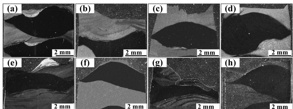
**Figure 9.** Fracture location in the samples tested along the Z direction: (a) without annealing, annealed at: (b) 500 °C; (c) 600 °C; (d) 700 °C; (e) 800 °C; (f) 900 °C; (g) 1000 °C; (h) 1100 °C.
