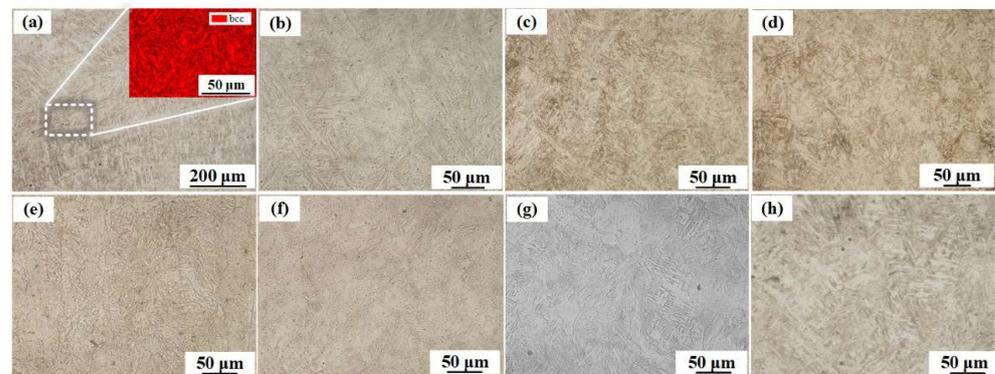
**Figure 4.** Microstructures of SS layer: (a) without annealing; (b) annealed at 500 °C; (c) annealed at 600 °C; (d) annealed at 700 °C; (e) annealed at 800 °C; (f) annealed at 900 °C; (g) annealed at 1000 °C; (h) annealed at 1100 °C.
