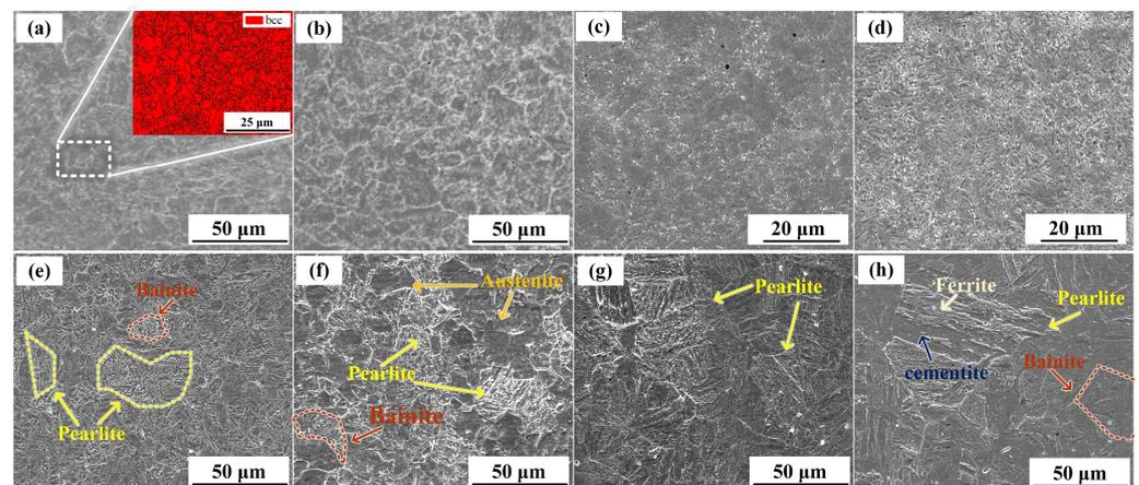
**Figure 3.** Microstructures of LCS layer: (a) without annealing, (b) annealed at 500 °C; (c) annealed at 600 °C; (d) annealed at 700 °C; (e) annealed at 800 °C; (f) annealed at 900 °C; (g) annealed at 1000 °C; (h) annealed at 1100 °C.
