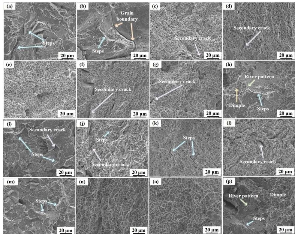
**Figure 8.** Fracture morphology in the Y direction: (a) without annealing; annealed at: (b) 500 °C; (c) 600 °C; (d) 700 °C; (e) 800 °C; (f) 900 °C; (g) 1000 °C; (h) 1100 °C; Fracture morphology in the Z direction: (i) without annealing; annealed at: (j) 500 °C; (k) 600 °C; (l) 700 °C; (m) 800 °C; (n) 900 °C; (o) 1000 °C; (p) 1100 °C.
