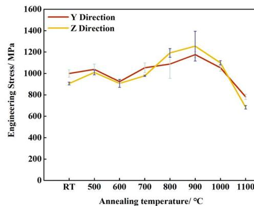
**Figure 7.** Tensile results in different annealing temperature.
