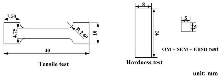
**Figure 2.** Dimensions of the testing specimens (unit: mm).
