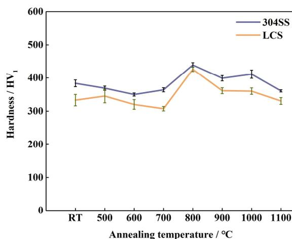
**Figure 10.** Hardness of 3304SS and LCS layers at different heat treatment temperatures.
