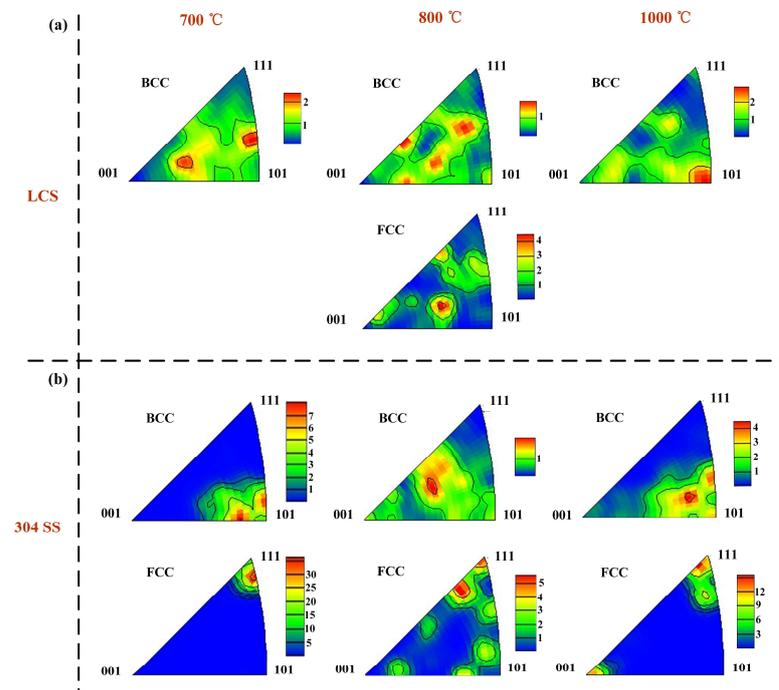
**Figure 6.** (a) Inverse pole figure of LCS in different annealing temperature; (b) Inverse pole figure of SS in different annealing temperature.
