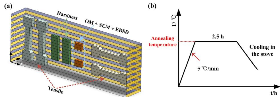
**Figure 1.** (a) Experimental set-up for the WAAM process and the Test sampling diagram; (b) Heat treatment process.
