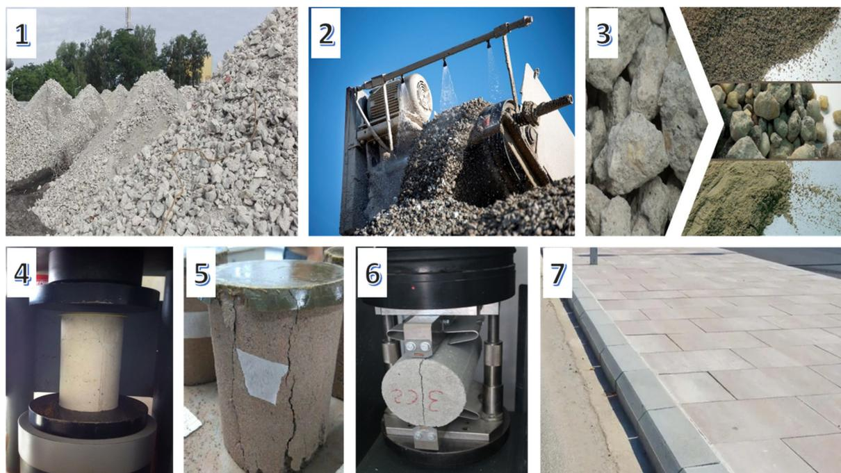
**Figure 1.** General procedure. (1) CDW selection. (2) CDW pretreatment. (3) Recycled aggregates. (4) Concrete testing specimen. (5) Characteristic prismatic fracture after compressive strength test. (6) Characteristic longitudinal fracture after tensile-splitting-strength method. (7) Industrial precast concrete pavement.
