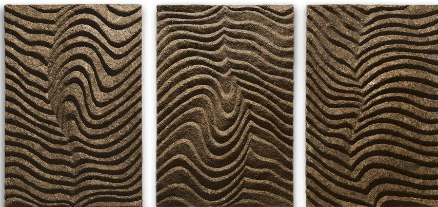
**Figure 3.** Sound absorption material from fillers (flax fiber and moss) with sapropel as a binder.
