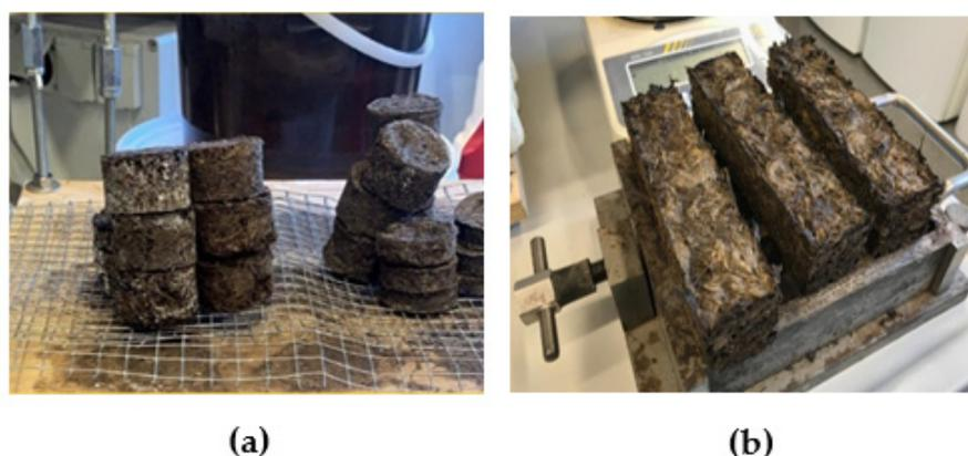
**Figure 2.** Developed material samples: (a) Samples for sound absorption and microbiological resistance tests; (b) Samples for mechanical strength tests.
