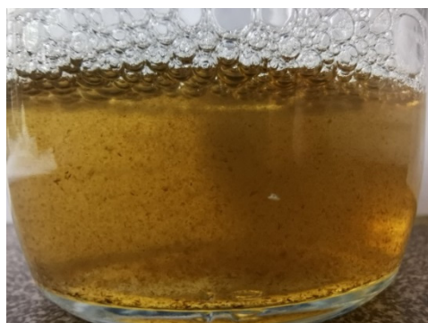
Figure 1. Visible aggregates of GO in RAE liquid medium (at pH = 4.1).
