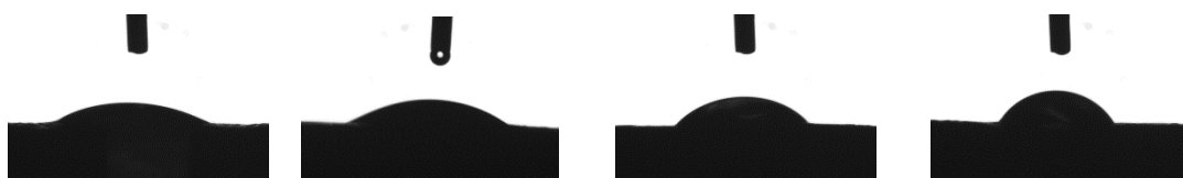
Figure 12. Illustrative microphotographs taken during the contact angle measurement. From the left, sBC, sBC_10/2, sBC_25/2, and sBC_50/2.
