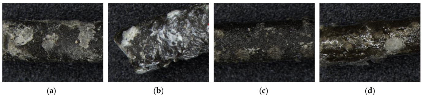
Figure 4. Surface condition of MPA: (a) unmodified, (b) modified with CA1, (c) modified with CA2, and (d) modified with CA3.
