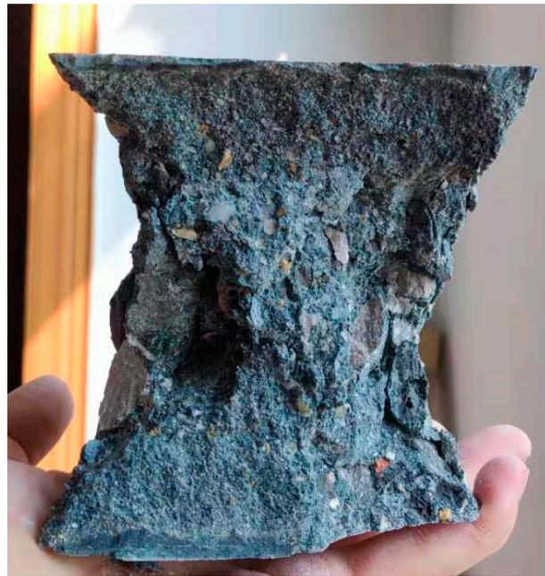
**Figure 6.** Concrete failure characteristics.
