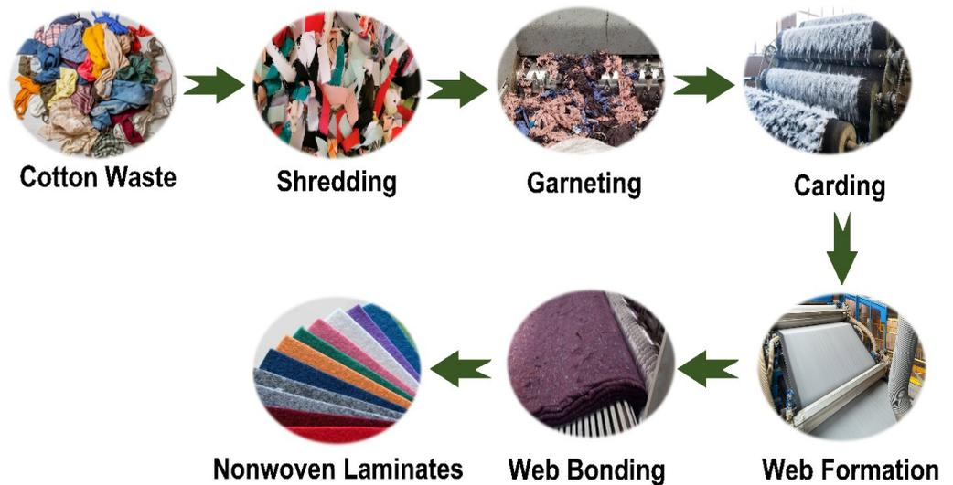
Figure 1. Illustrative process sequence to fabricate nonwoven laminates utilizing CW.
