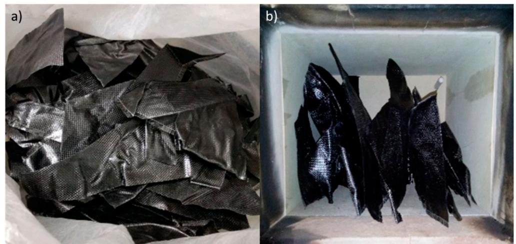
Figure 1. Scraps of prepreg 8552/AS4 plain-wave (Hexcel) (a) as received and (b) as placed into the furnace.
