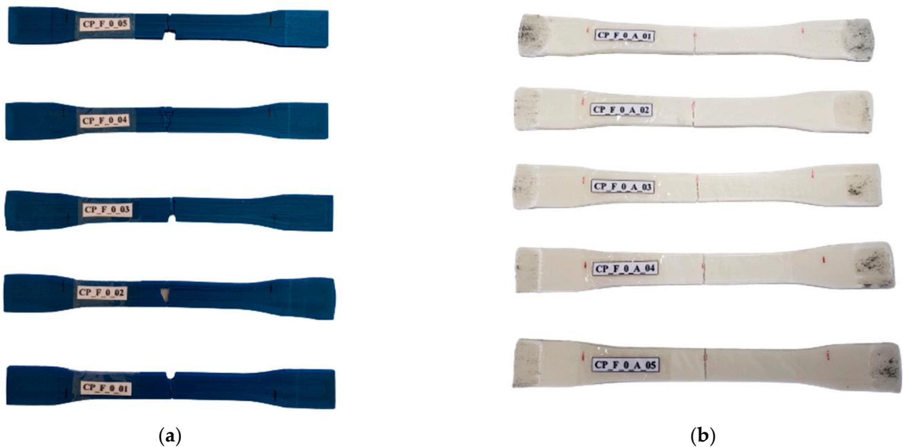
**Figure 4.** Specimens 3D-printed under flat orientation after tension testing: (a) specimens in PET-G and (b) specimens in ABS.
