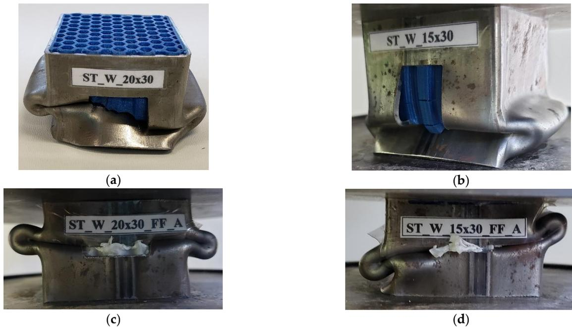
**Figure 8.** Deformed specimens after axial compression (a,b) PET-G (c) and (d) ABS.
