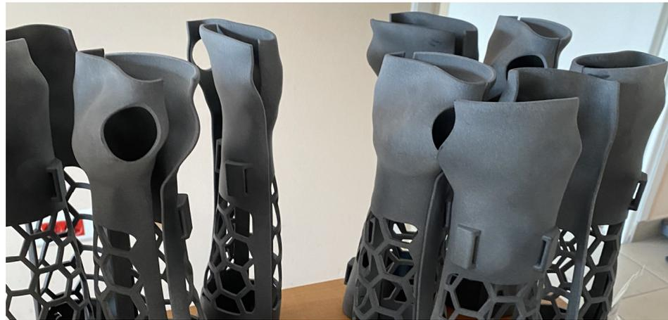
**Figure 13.** Forearm orthoses production example made in HP MJF technology.
