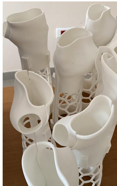
**Figure 14.** Forearm orthoses production example made in SLS technology.
