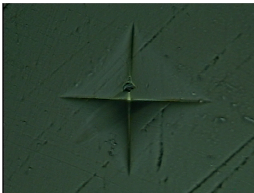
Figure 7. One typical indentation point of cryogenically cooled PMMA under a microscope.
