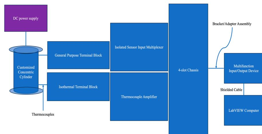
**Figure 10.** Schematic diagram of thermal conductivity measurement of MS nanofluids.
