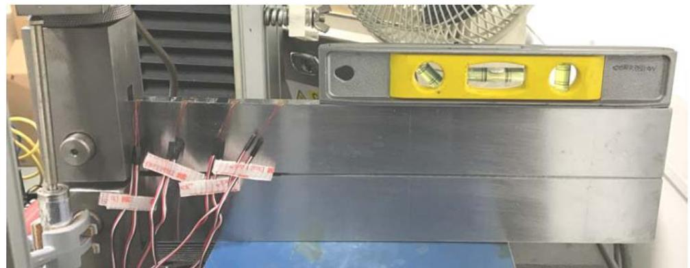
Figure 24. Large-scale DCB specimen from experiment by Maldonado [178] (the width and side notch dimensions were maintained within the NACE TM0177 limits, while all other dimensions were scaled up by a factor of 3.9x).
