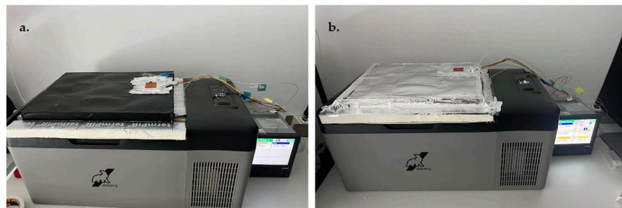
**Figure 6.** Test stand for measuring thermal properties of structured panels with the geometry of the inner core of the gyroid made using 3D SLA technology; (a) four-layer panel with outer black polyethylene film, (b) four-layer panel with outer metallized polyethylene film (elaborated by authors).
