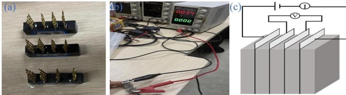
**Figure 3.** (a) Schematic diagram of resistivity test sample, (b) schematic diagram of voltage regulator power supply, and (c) schematic diagram of resistivity test principle.
