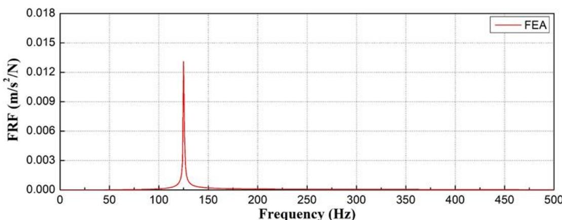
**Figure 11.** Analyzed natural frequency of concrete sleeper with normal condition.
