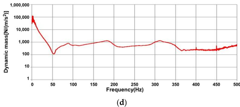
**Figure 8.** Dynamic mass prediction results. (a) Undamaged concrete sleeper; (b) Crack #1; (c) Crack #2; (d) Crack #3.
