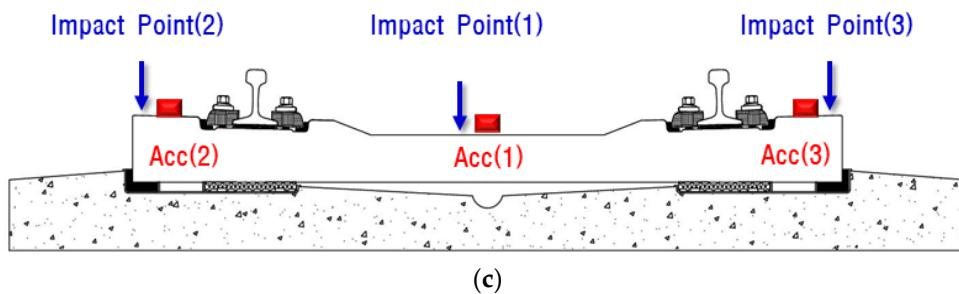
**Figure 2.** Photographs of modal test using impact hammer. (a) Overview of test track; (b) impact hammer test; (c) schematic of instrumentation.
