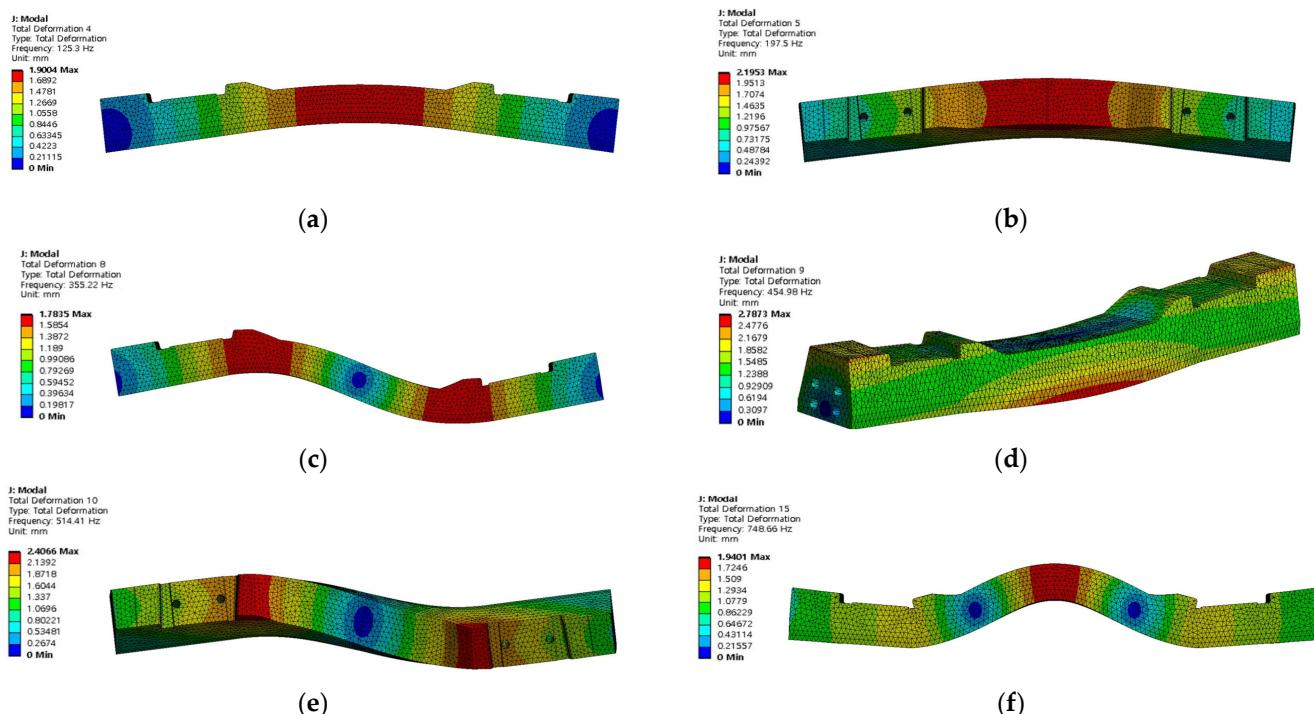
**Figure 10.** Analysis results (mode shape). (a) 1st mode (125.30 Hz); (b) 2nd mode (197.50 Hz); (c) 3rd mode (355.22 Hz); (d) 4th mode (454.98 Hz); (e) 5th mode (514.41 Hz); (f) 6th mode (748.66 Hz).
