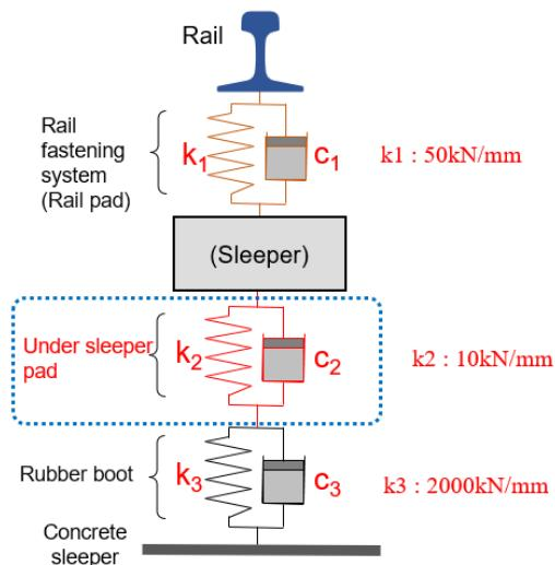
**Figure 4.** Concrete sleeper spring model.
