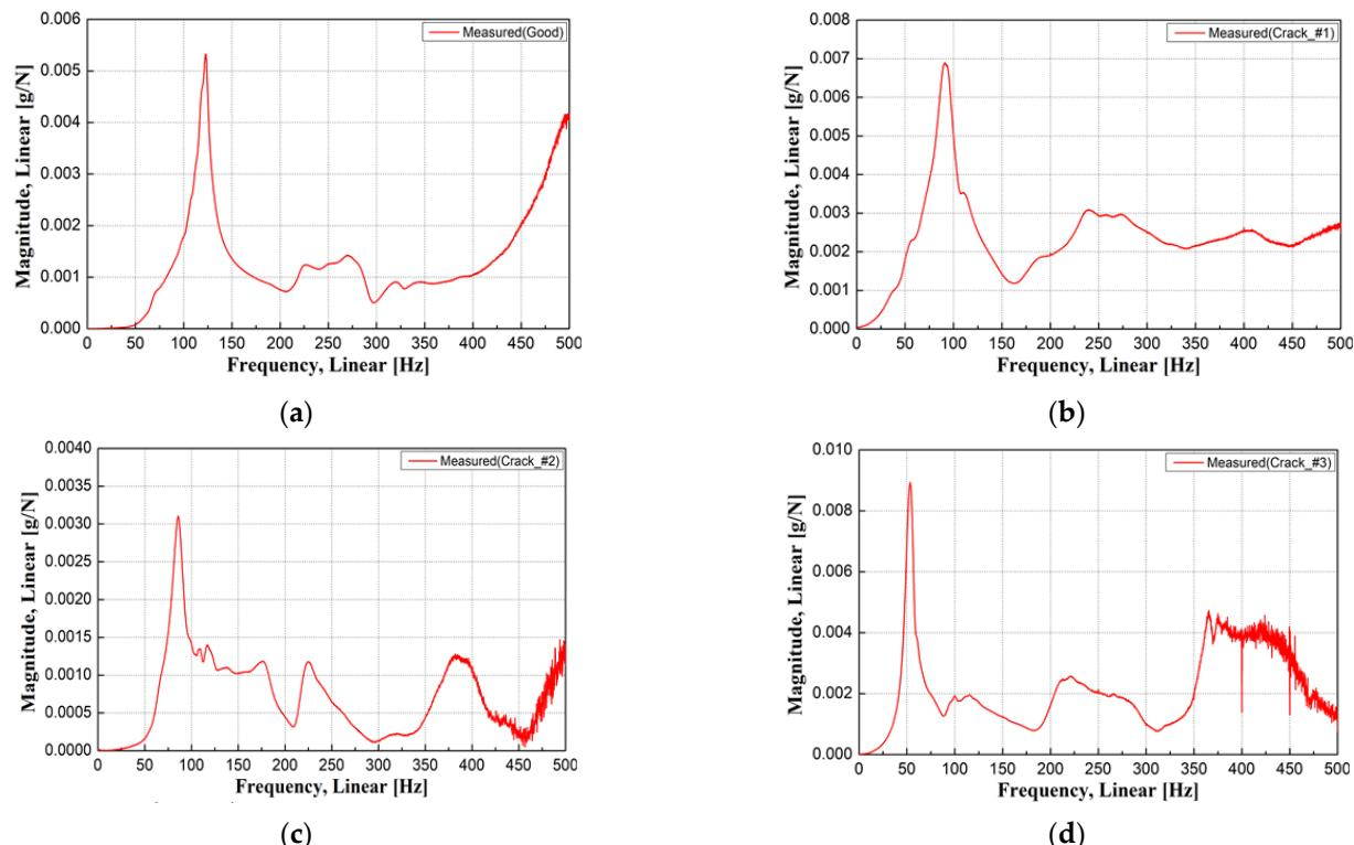
**Figure 7.** Measurement results of frequency response function (FRF) for each sleeper. (a) FRF (good); (b) FRF (Crack #1); (c) FRF (Crack #2); (d) FRF (Crack #3).
