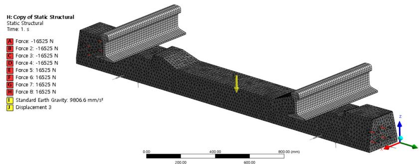
**Figure 5.** Post-tensioning concrete sleeper modeling.
