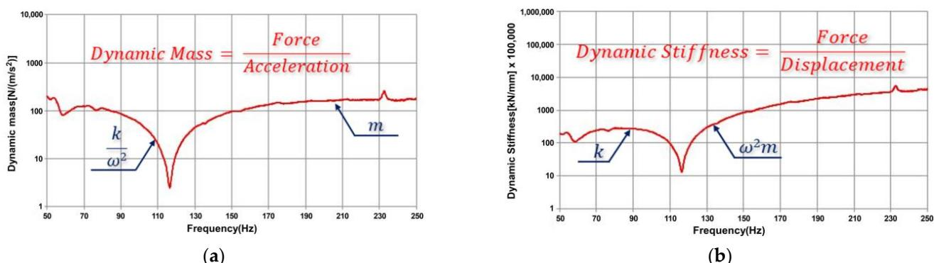
**Figure 3.** Dynamic mass-and-stiffness estimation of single degree of freedom. (a) Dynamic mass ( $m$ ); (b) dynamic stiffness.
