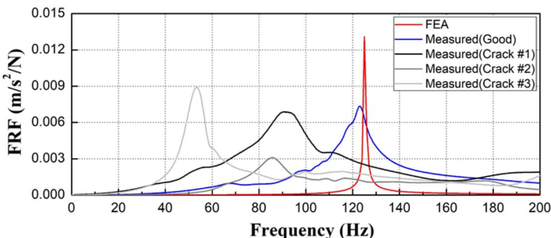
**Figure 13.** Comparison of modal test and numerical analysis results.
