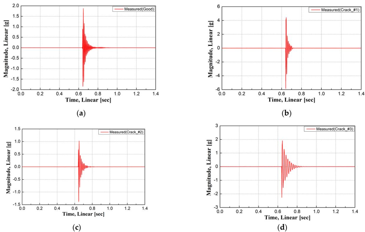
**Figure 6.** Measurement results of dynamic response function (FRF) for each sleeper. (a) Time acceleration (Good); (b) time acceleration (Crack #1); (c) time acceleration (Crack #2); (d) time acceleration (Crack #3).
