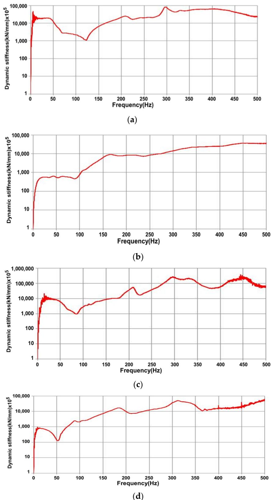
**Figure 9.** Dynamic stiffness prediction results. (a) Undamaged concrete sleeper; (b) Crack #1; (c) Crack #2; (d) Crack #3.
